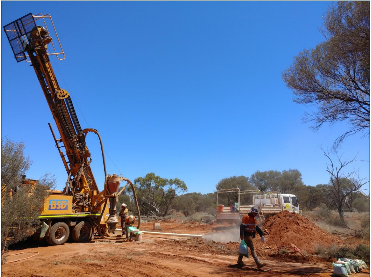
Figure 2. RC drill rig on site collaring first hole at Mt Venn
