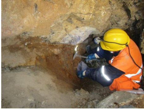
Figure 3: LEFT Preparing channel sample IM-001077 at Wari. The photo shows a 0.5m wide mineralised vein that is highly ferruginous which makes it red-brown in appearance (similar to the Vilcapuquio breccia veins). IM-001077 contains visible galena and smithsonite and has returned grades of 31.34% Zn, 184g/t Ag and 21.00% Pb.
