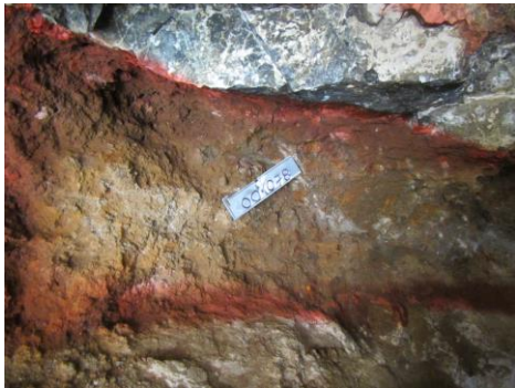
Figure 4: LEFT Location of channel sample IM-001078 at Wari. The photo shows a 0.3m wide mineralised vein that is highly ferruginous (as for IM-001077). IM-001078 contains visible galena and smithsonite and has returned grades of 33.76% Zn, 169g/t Ag and 17.33% Pb.
