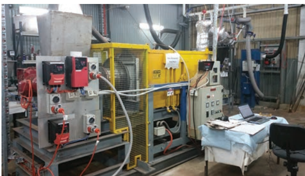
Figure 8.2: Barite pre-flotation circuit at ALS test facility in Perth, Western Australia.
