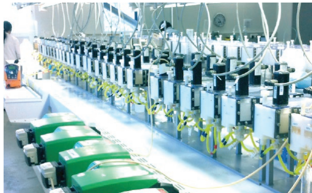
Figure 8.4: Solvent Extraction test facility at ANSTO Minerals.
