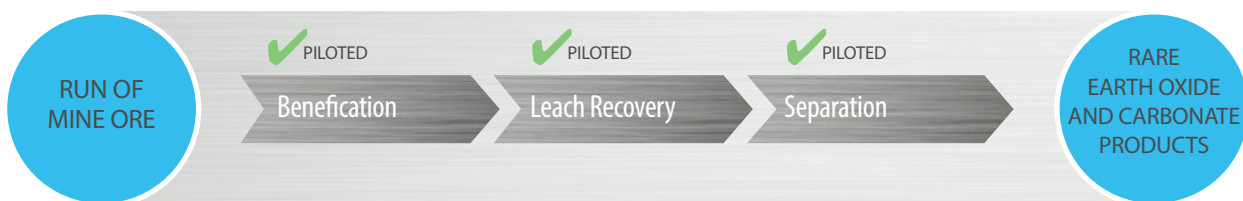
Figure 8.1: Simplified summary of the three stage process developed by Peak for Ngualla's rare earth mineralisation.
