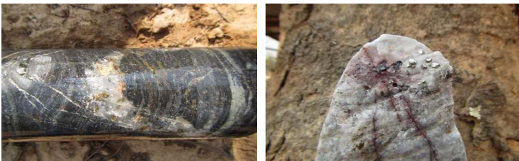
Examples of visible chalcopyrite mineralisation intersected in DKAT_DD01 at Katete
