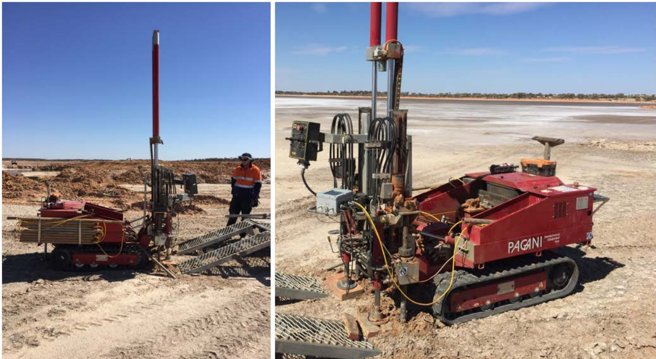
Figure 4: Cone Penetrometer Rig in Operation on Lake Wells
