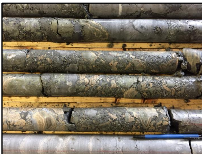
Figure 4: Colloform and brecciated massive sulphides comprising sphalerite (tan), marcasite (greenish), and galena (metallic grey) from the Base of Reef intercept in Z_4069_008.
