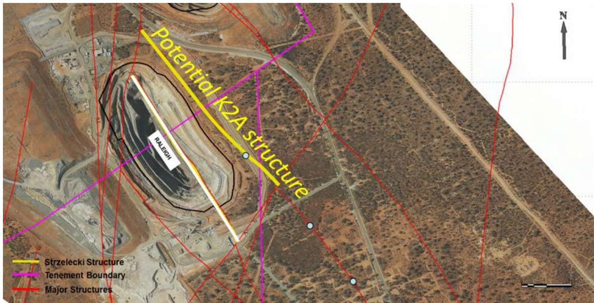
Figure 4. Aerial photograph of Raleigh pit and surrounds showing major structures and secondary footwall K2A structure tested in-mine during quarter one.
