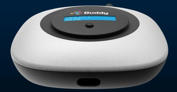
Buddy Ohm measures electricity, gas, water and steam consumption, along with solar generation + temperature/humidity via small remote sensors
