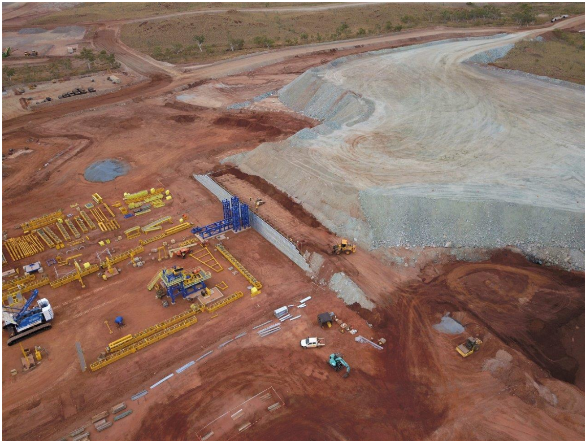
Aerial view of ROM pad and primary and secondary crushing circuit
