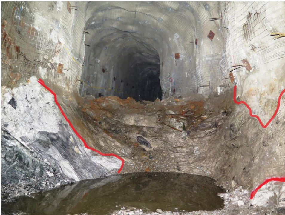
385 SOD bench showing massive ore with a face grade of 6.5% nickel
