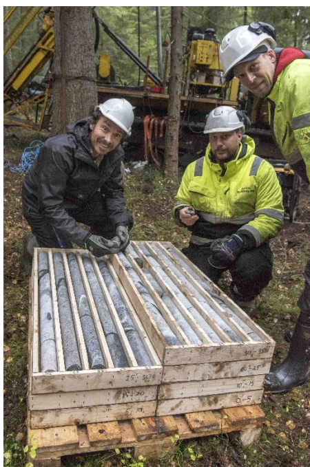
Figure 3 | Drilling at Middagshville Cobalt Mine region, recently drilled core at the rig, and core trays delivered to the logging room
