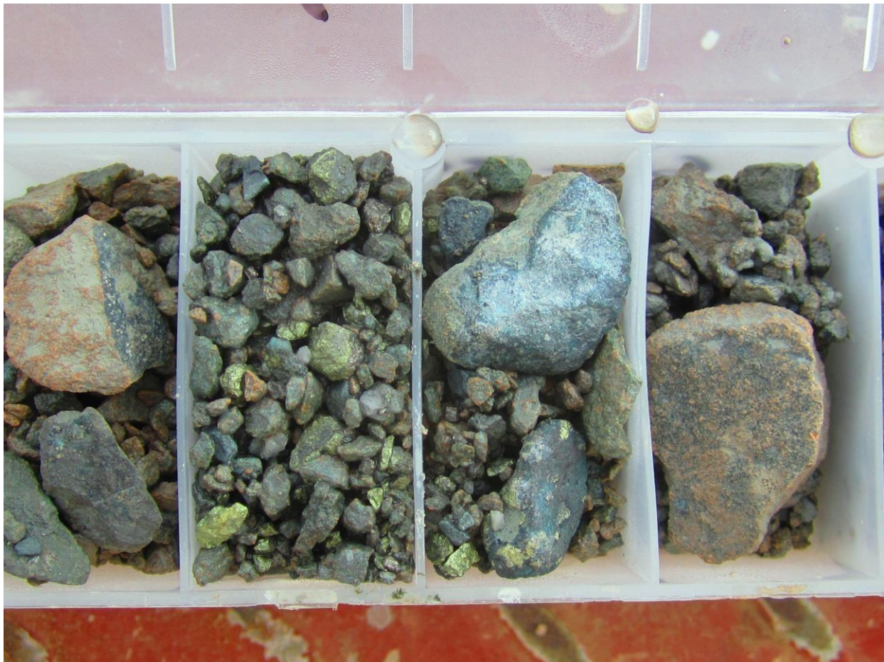
Abundant chalcopyrite mineralisation in drill hole DDRC011 from 74-75m.
