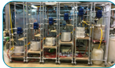
Neutralisation & Precipitation Circuit
