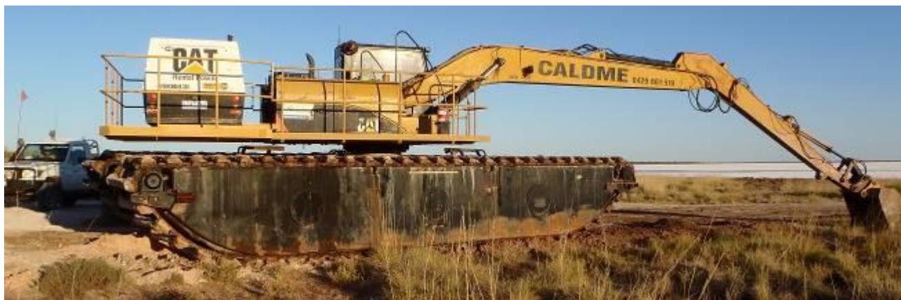
Figure 8 Amphibious Digger with Air Lift Compressor
