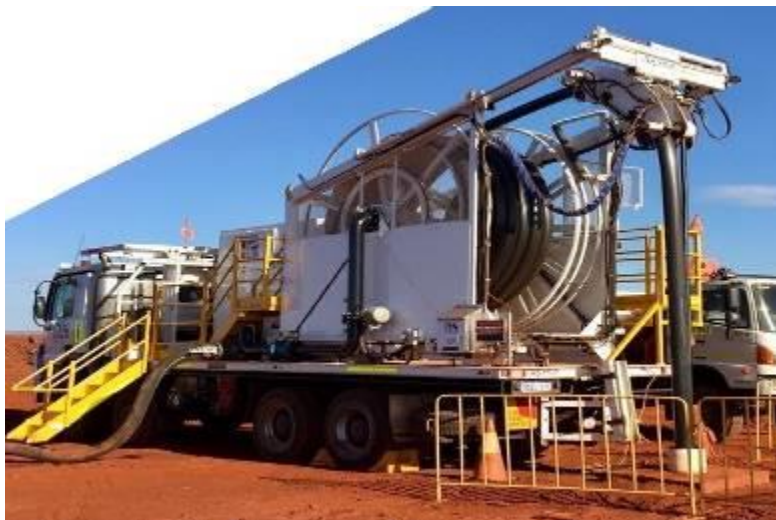
Figure 6 An example of test pumping in a Process Water Borefield (not at LD)
