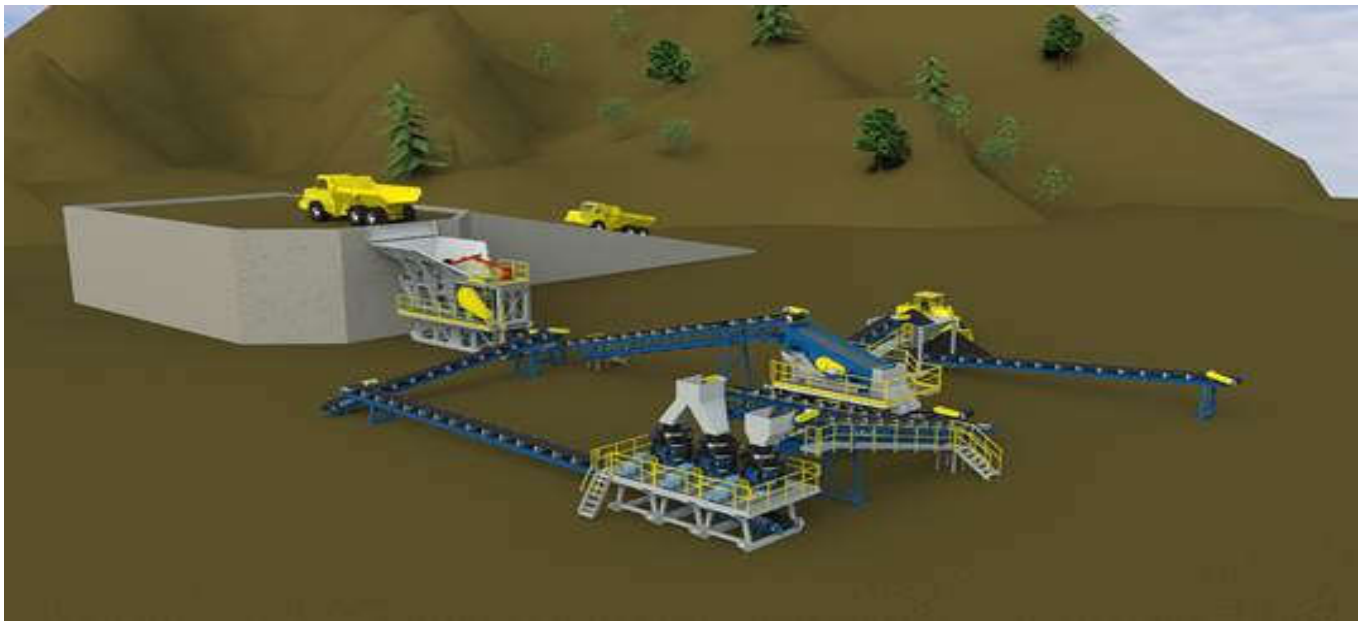
Figure 5: Sepro Systems 75t/h three stage crushing circuit
