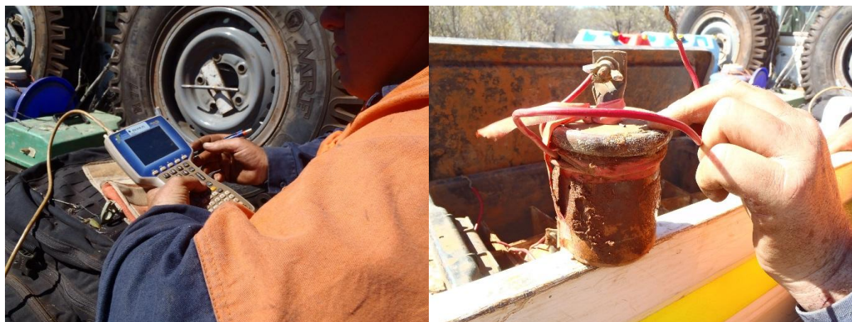
Figure 5– Field measurements using porous pot electrodes (right) during the September gradient-array induced polarisation surveys at the Ngalia Regional project.
