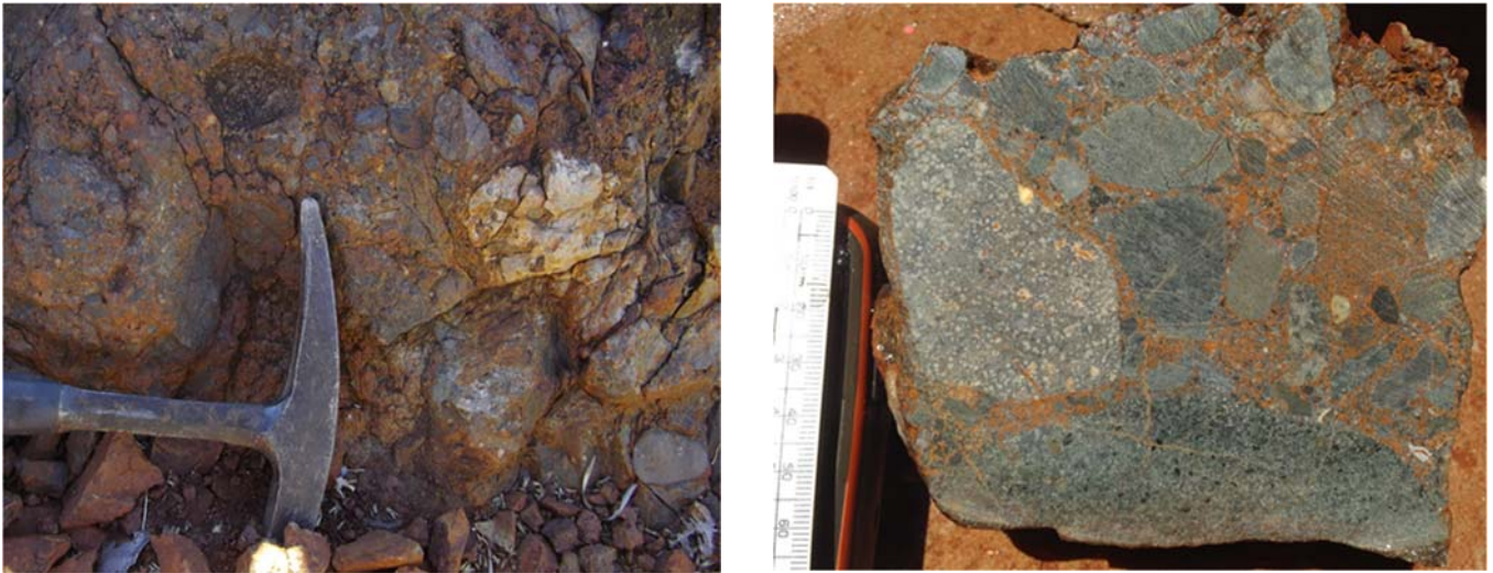
Figure 5 Jarret Well upper conglomerate in outcrop (left) and cut hand specimen (right) showing rounded to angular volcanic clasts and fine matrix with minor pyrite and limonite and hematite after pyrite.
