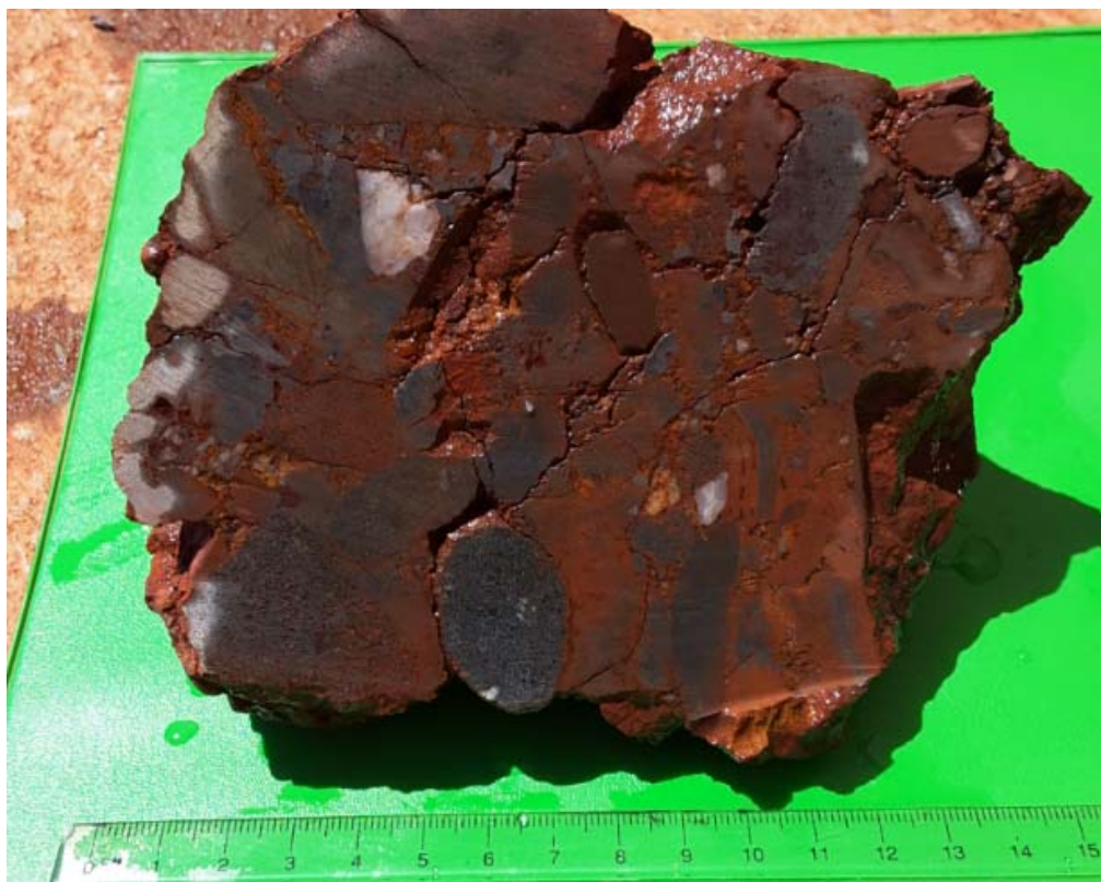
Figure 3 Jarret Well lower conglomerate showing ferruginous matrix after pyrite.
