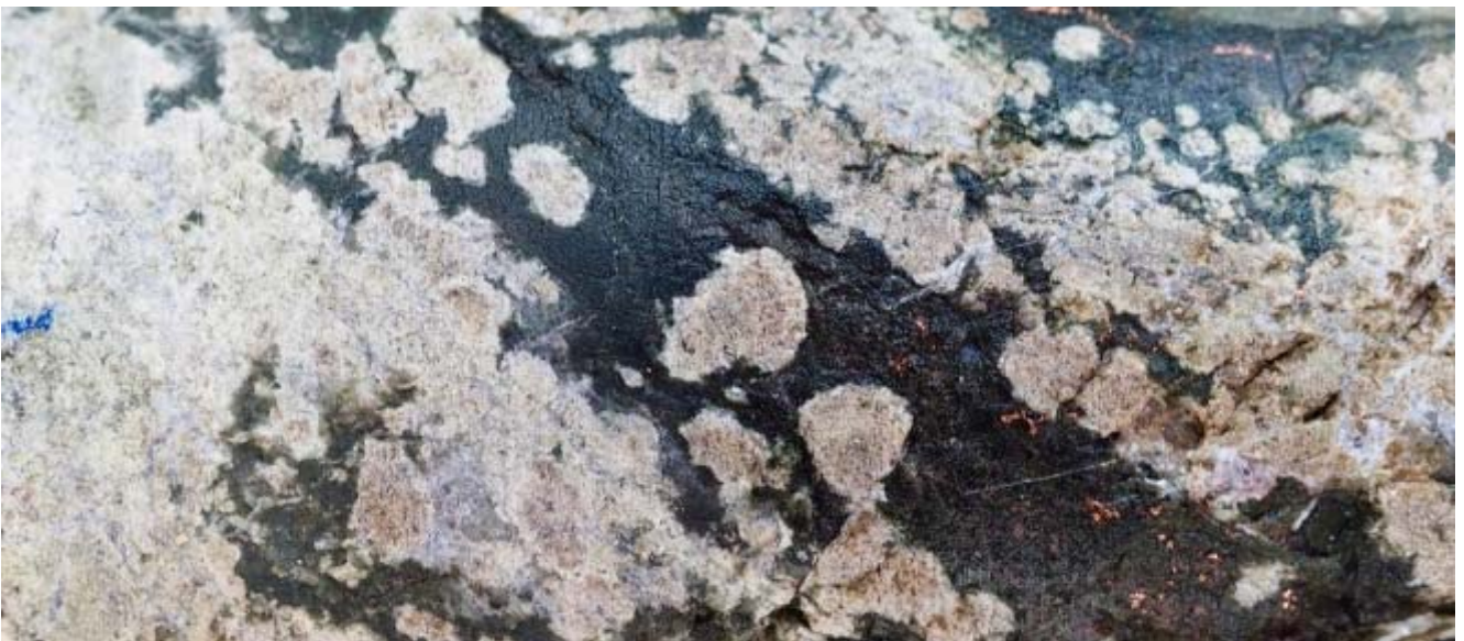
Figure 6 Finely disseminated Native Copper in red and green garnet skarn, ZM17010 153.7m
