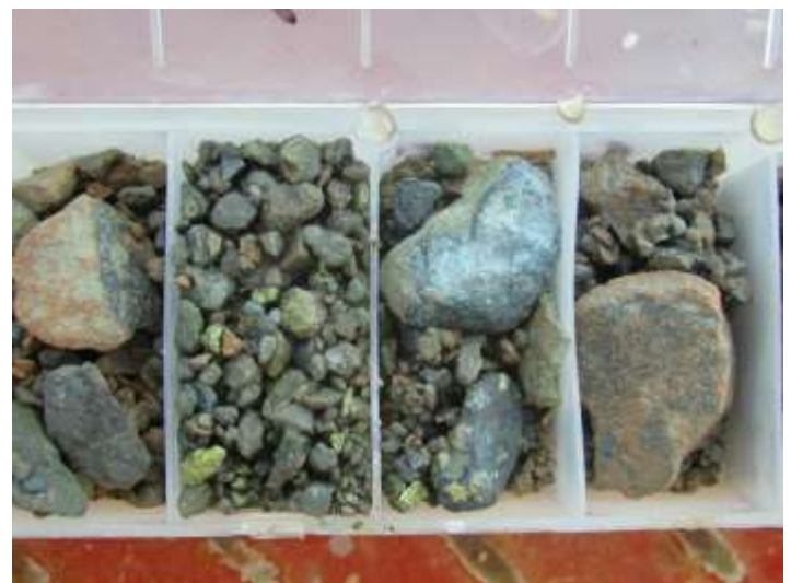
Photo 1. Cobalt mineralisation occurs as black spots of siegenite, a Co-Ni sulphide, in sandstone and siltstone layers – is from drill hole DD17RC010 44-46m. Photo 2 Chalcopyrite mineralisation in drill hole DDRC011 from 73-75m. The abundance is estimated at ~5-10% chalcopyrite.
