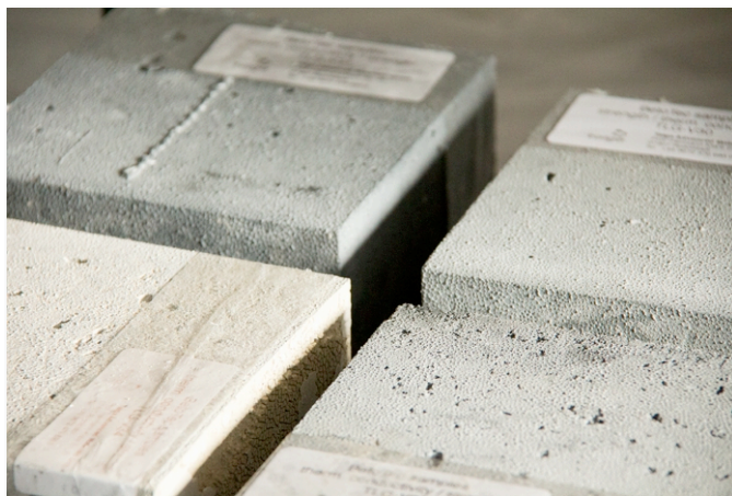
Figure 1. Thermally conductive concrete test samples using Talga graphene and graphite products.
