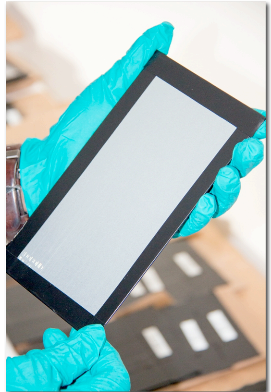
Figure 5. Talga transparent graphene-based coating on steel test panel.
