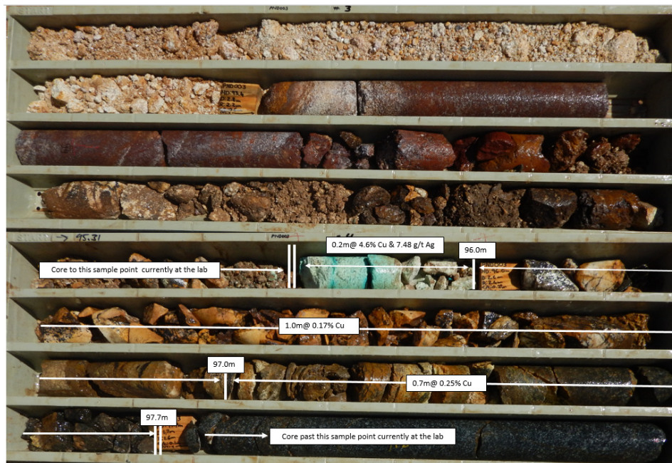
Figure 12: Drill core from PND003 showing the supergene zone, chrysocolla occurrence and zones where additional assaying is currently in progress
