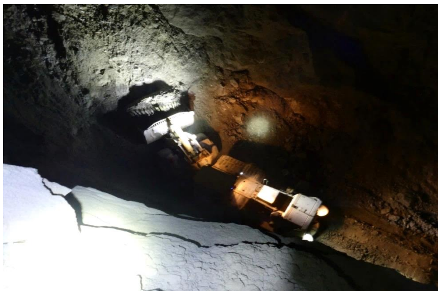
Figure 5. View from 1394 Level of the Tele Remote Control Bagger loading Ore in the Long Hole Stope on the 1380 Level at the A1 Gold Mine
