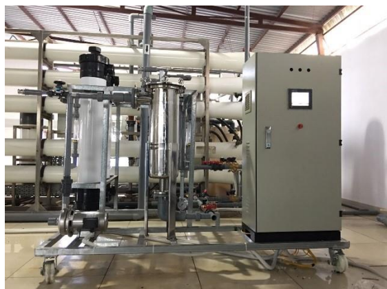
Picture: Pilot Water Treatment System using De.mem membranes deployed in Vietnam
