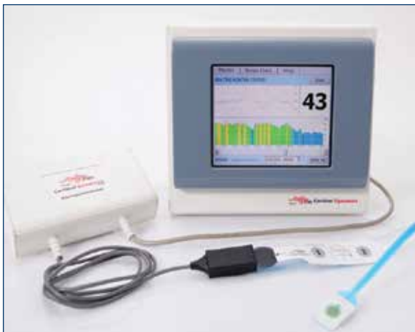
Cortical's Brain Anaesthesia Response (BAR) Monitor.
