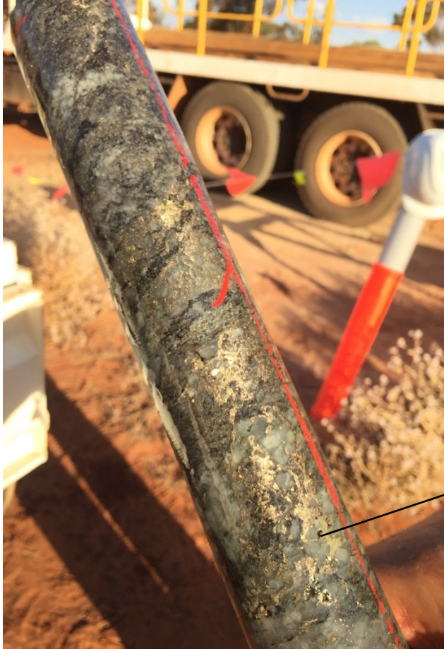
Pyrrhotite & pyrite in altered gneiss: RDH04 153-157m 15.20g/t
