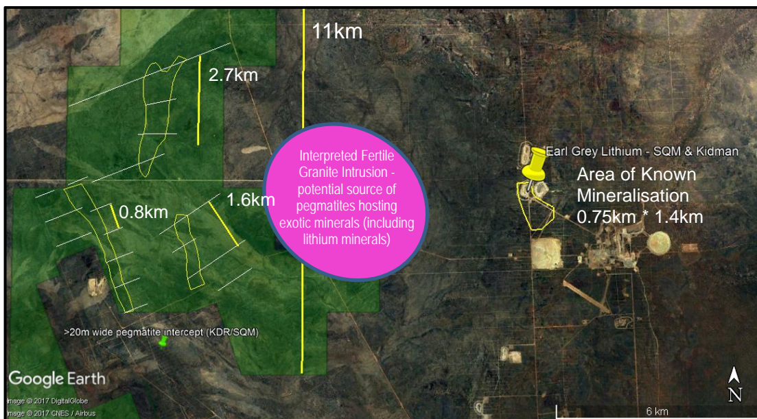
Figure 2: White lines represent location of 1st phase of RAB drilling, shaded green area is Hannans tenement E77/2219, green ellipse is lithium anomalism from 1st phase of RAB drilling, pink oval shape is cartoon only of interpreted granite, yellow lines are 'distance/length' markers.
