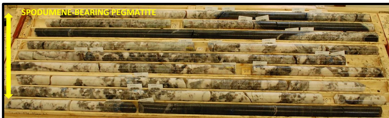
Figure 6. Drill core obtained from drill hole SL-17-54 (core from 76.2m to 88.6m) showing the intersection of high-quality spodumene-bearing pegmatite (the lighter coloured material in the photo is the Pegmatite, whilst the darker material is Mafic Volcanic).
