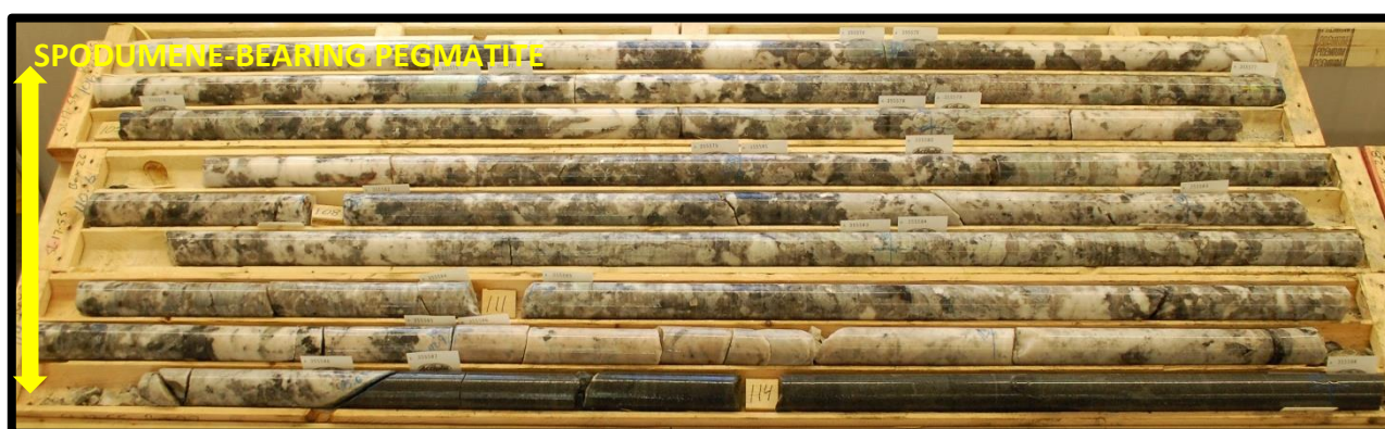
Figure 7. Drill core obtained from drill hole SL-17-55 (core from 102m to 114.7m) showing the intersection of high-quality spodumene-bearing pegmatite (the lighter coloured material in the photo is the Pegmatite, whilst the darker material is Mafic Volcanic).
