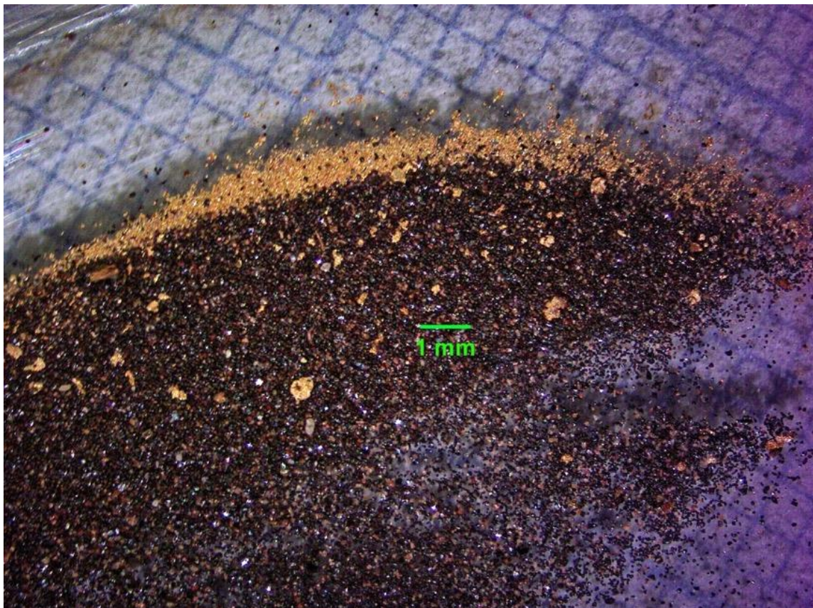
Figure 5: Fine gold particles panned from a grab sample near the base of the second conglomerate horizon exposed in trench 2. Most of the gold particles along the top edge of the image are less than 100 microns across.
