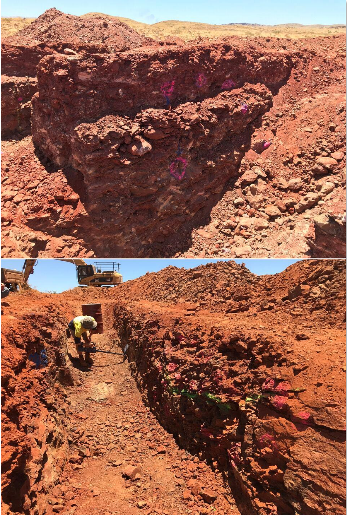
Figure 2: Top, photograph of a pit wall in trench 3. From the floor of the pit to the top of the bench is approximately 2.5 meters. Boulders and cobbles comprising the conglomerate are evident in the pit wall. Small pink paint spots mark metal detector strikes in bedrock. Bottom, photograph looking down the length of trench 7. A geologist uses a metal detector to locate strikes. The basal contact of a conglomerate bed is marked with green paint. A steel sample drum and the 40-tonne excavator used for trenching are in the background.
