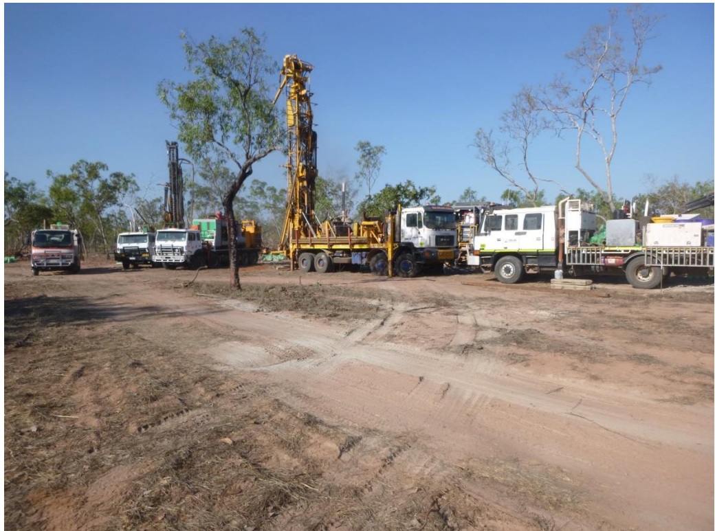
Two RC drill rigs resource drilling at the Stanton Cobalt Deposit
