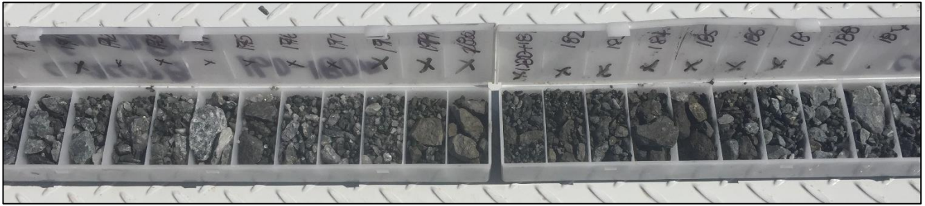
Photo 1: Mineralised zone in CORC078 returning 10m @ 1.4% Cu, 1.1% Zn and 0.15g/t Au from 178m
