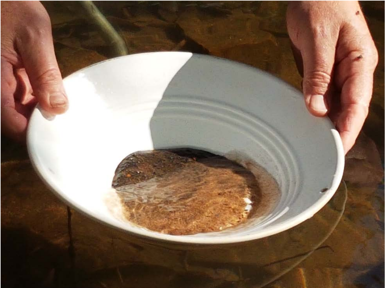
Figure 9. Pan concentrate from the Buldiva prospect area, with abundant cassiterite (black grains).
