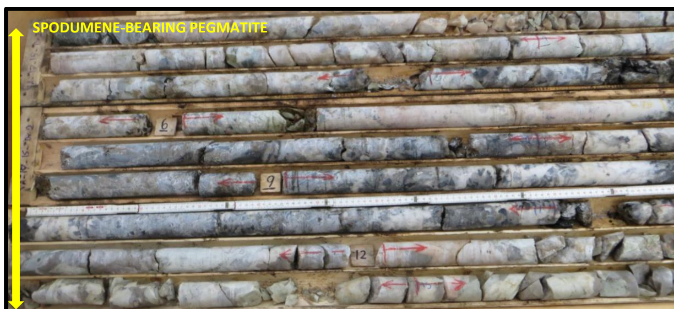
Figure 1. Drill core obtained from drill hole SA-17-15 showing the intersection of a portion of high-quality spodumene-bearing pegmatite from 2m down hole (the lighter coloured material in the photo is the Pegmatite, whilst the darker material is Mafic Volcanic).
