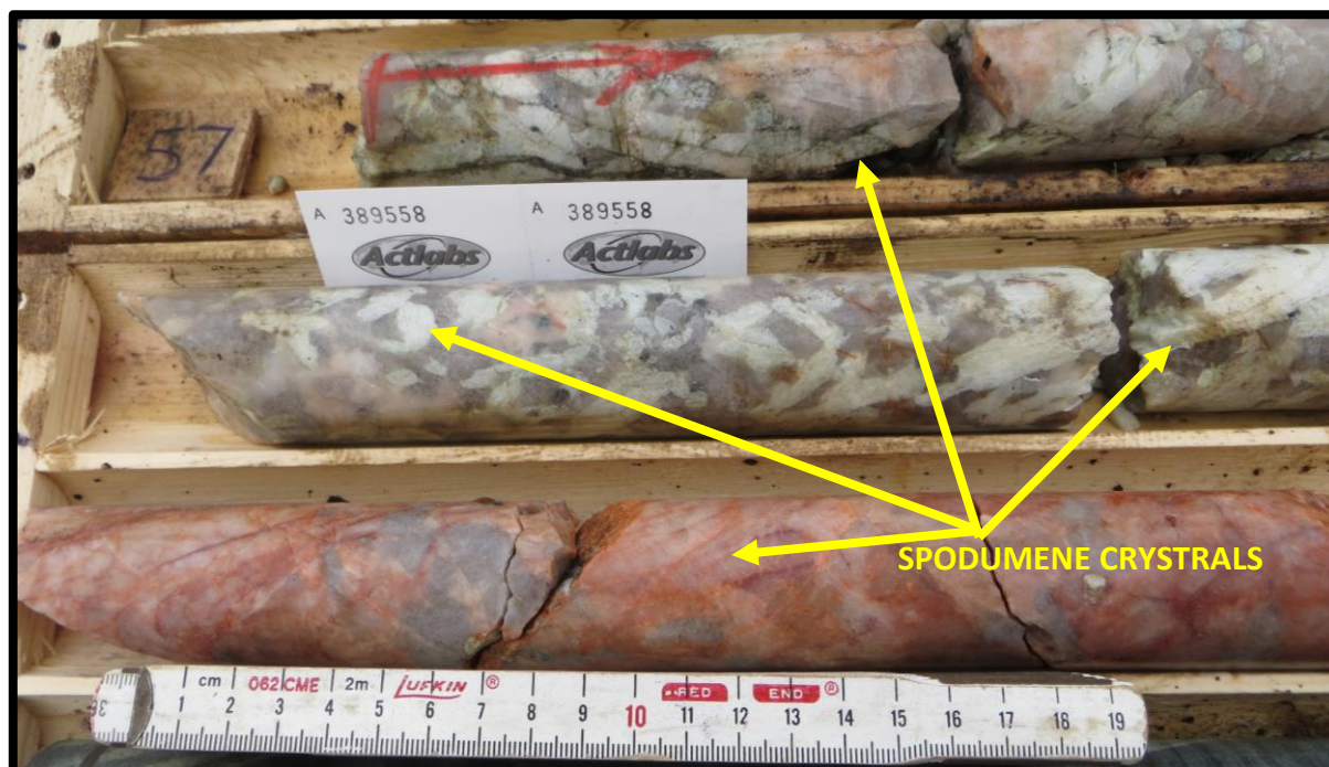
Figure 4. Image of very large white and red spodumene crystals from drill core SA-17-07 showing a portion of core from 57m down hole.
