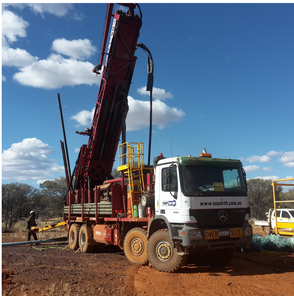
Figure 2: RC Drill rig at Kyarra Cobalt project
