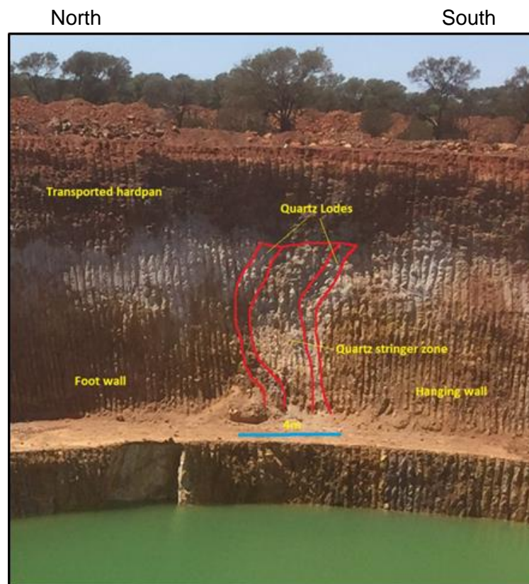
Figure 4. Photo of Eastern Wall of Mixy Trial pit and positions of the Main Zone gold veins and inter-vein alteration and quartz stringer zone. Blue bar is ~4m.
