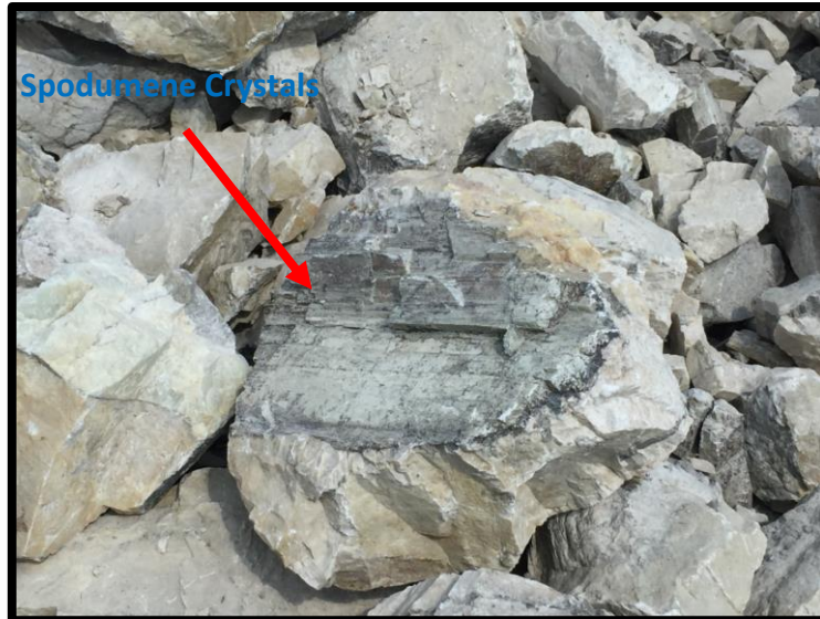
Figure 1. Bulk sample of Spodumene bearing pegmatite obtained from the North Aubry prospect.
