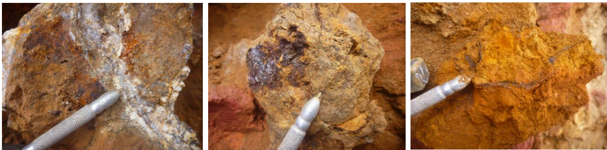
Figure 3: ABOVE LEFT Smithsonite /galena veinlet (IM-000325: 2.98% Zn, 80.5g/t Ag, 3.95% Pb); ABOVE MIDDLE Fe-oxide rich mineralisation (IM-000324: 4.52% Zn, 30.1g/t Ag, 1.54% Pb); ABOVE RIGHT Highly ferruginous boxwork gossan mineralisation (IM-000327: 106g/t Ag, 7.39% Pb); RIGHT A combination of veinlets with galena and boxwork gossan styles of mineralisation (IM-000337: 2.39% Zn, 58.5g/t Ag, 3.67% Pb).
