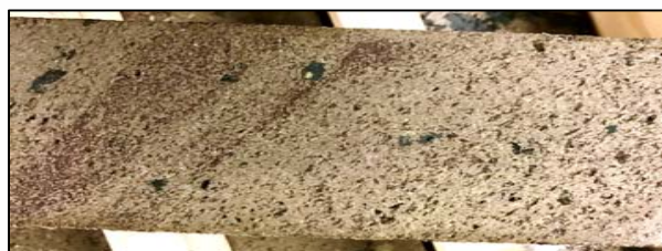
Sphalerite & pyrrhotite in SBJK170003 (14.71m @ 2.2% Zn, 1% Cu)
