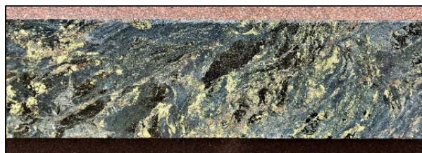
Chalcopyrite & sphalerite in SBJK170006 (24.4m @ 1.1% Cu)
