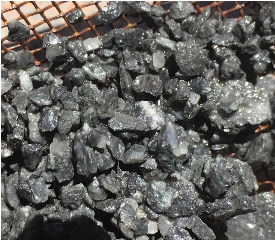
Figure 6: Close up of washed RC chips grading 6.86g/t Au and up to 15% arsenopyrite from hole KNC170039. Metallurgy confirms gold recovery, via gravity and standard cyanide leach, of over 94% with gold in fractures within and on the edges of the arsenopyrite.
