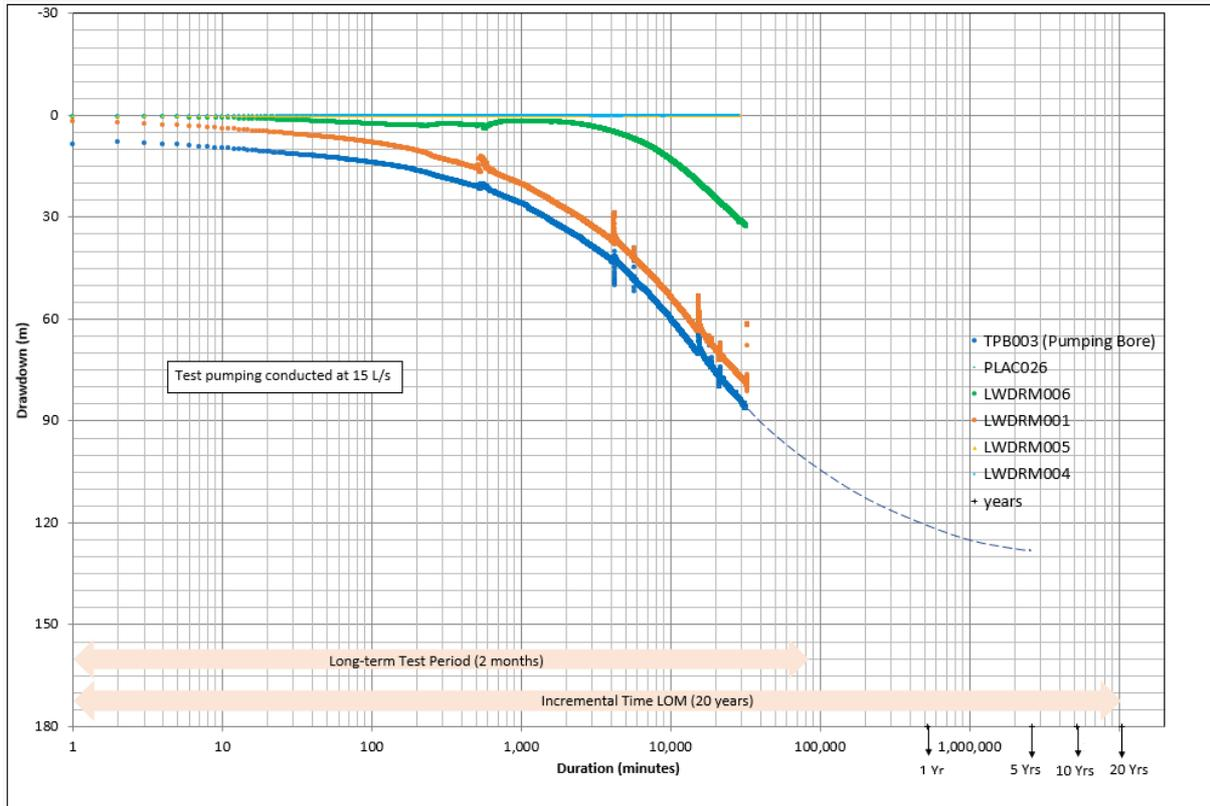
Figure 5: TPB003 Test Pumping Response
