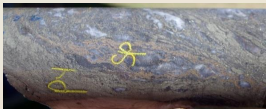
OFDD001: 246m (left) & 248.5m (right) drill core showing strong shearing, epithermal qtz veining, pyrite (py) & sphalerite (sp)
