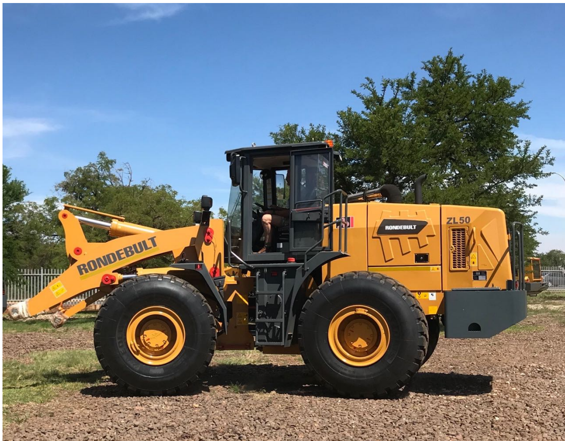
Figure 2: Newly purchased 5t loader for feeding the refurbished Graphmada Process Plant (without bucket).
