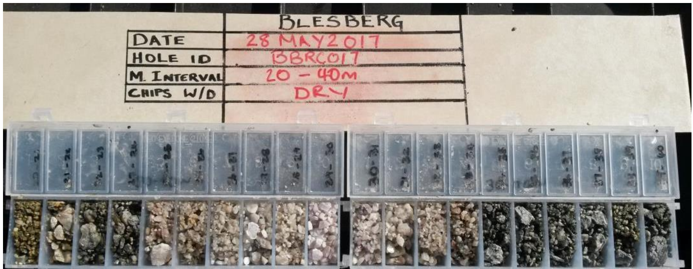
Plate 2. BBRC017 20-40m Chip tray. The pegmatite intercept is clearly identifiable within the country granodiorite by its white colour and abundance of feldspar, quartz \pm mica. Spodumene content is recorded up to a maximum of 50% (29-30m) in intervals 27-33m and corresponds with significant intercept, 2m @ 10,505ppm Li from 29m
