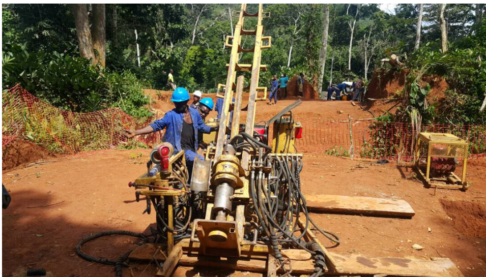
Figure 1: African Drilling Limited's Diamond Drilling Rig on site at Kabotshome Gold Prospect
