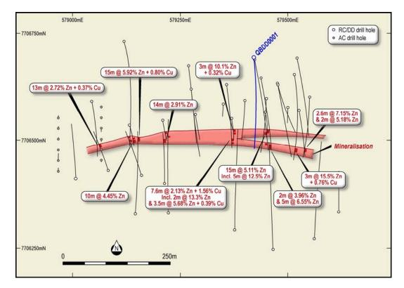
Figure 3. Drillhole location plan showing QBDD0001 and historical results.
