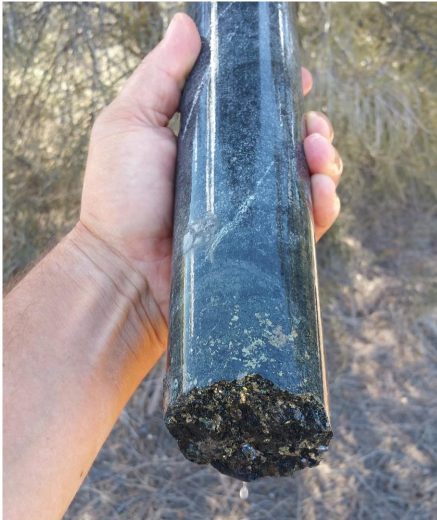
Figure 1. Photograph of a sulphide accumulation in NCB0003 from approximately 290m downhole.
