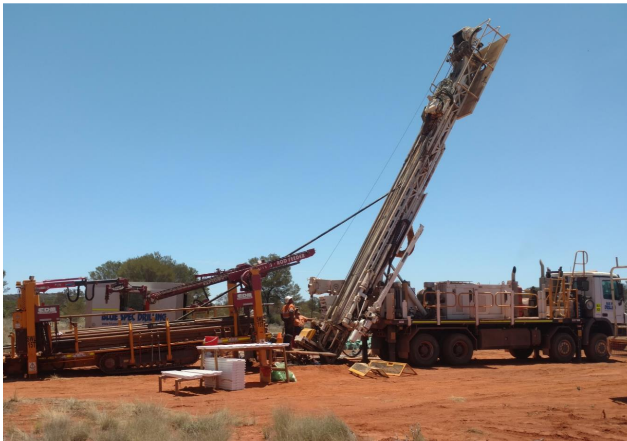
Diamond drilling underway at Mt Venn
