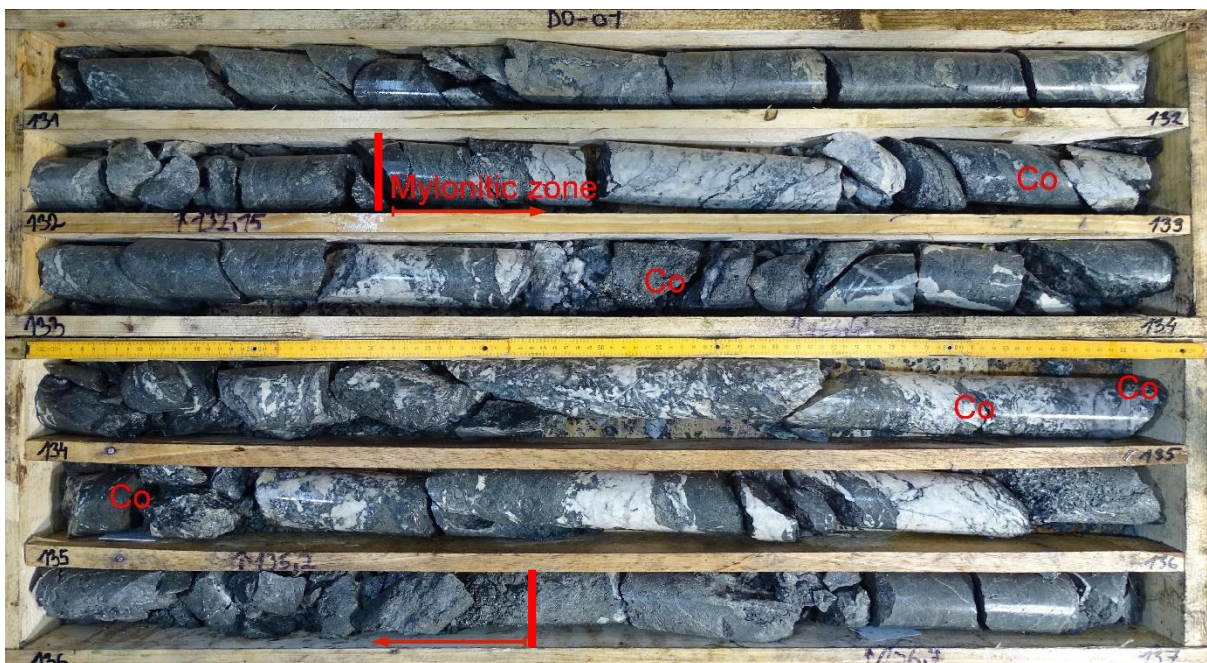
Figure 1: Mylonitic Zone Containing Disseminated to Blebby Cobaltite-Gersdorffite Sulphides & Zone of Semi Massive Cobalt-Gersdorffite Sulphides
