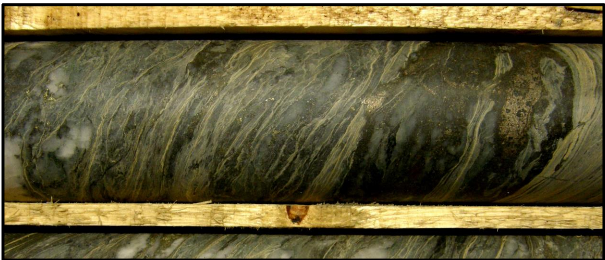
Photo 5 TIDD004 (162.2m): narrow zones of semi-massive and disseminated sulphide in a strongly sheared host rock, dominantly pyrrhotite and coarse grained pyrite with minor chalcopyrite blebs.
