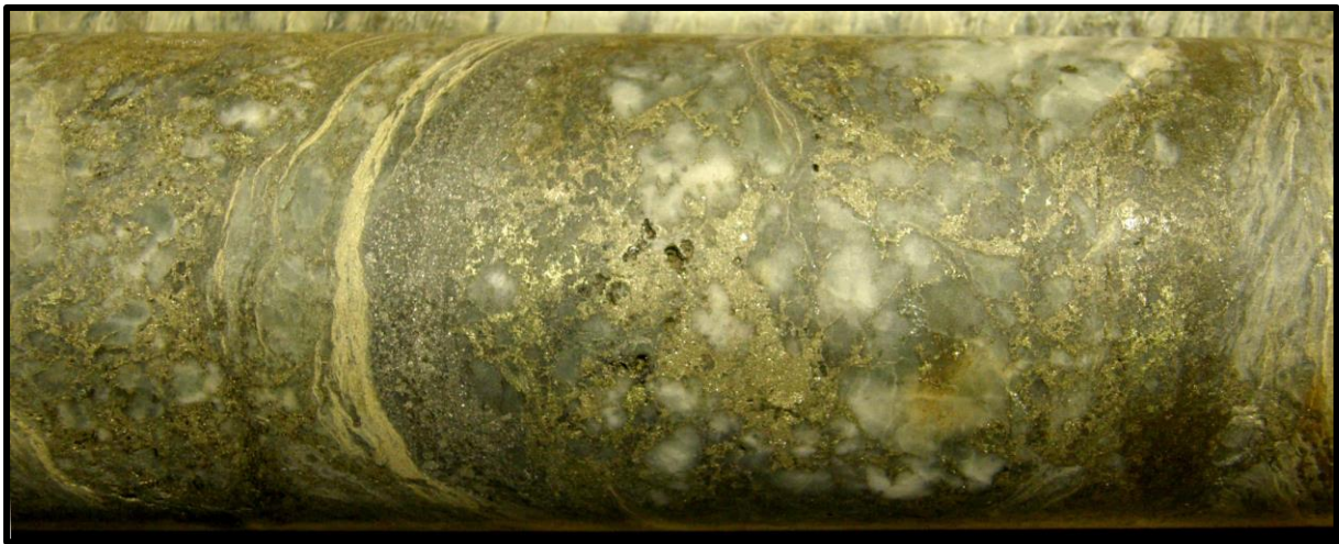
Photo 4 TIDD004 (161.8m): network textured sulphides, dominantly pyrrhotite and coarse grained pyrite with minor chalcopyrite blebs.
