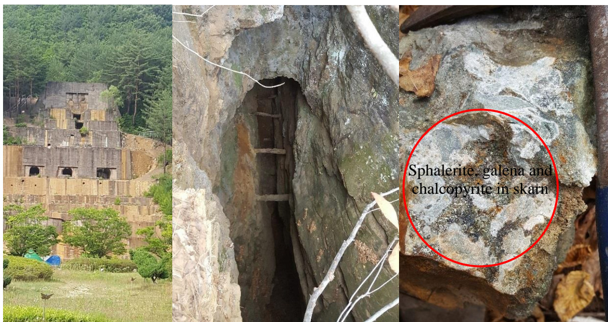
Photo's 1 – 3: Ilweol, historical processing plant, underground stoping and sulphides in skarnified limestone
