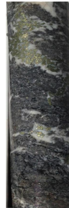
Drill core CCD02, mineralised evaporite horizon, disseminated chalcopyrite. Visible ex-gypsum crystals of evaporite horizon
